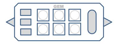
GEM can be used as a direct replacement for the 1.5" (38mm) long filament-lamp commonly found in automotive light fittings
