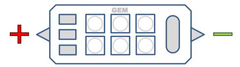
The contacts in the light fitting may require bending inwards slightly to hold the module firmly in place. When installing the module make sure that no parts other than the exposed end contacts touch any metalwork inside the fitting.
