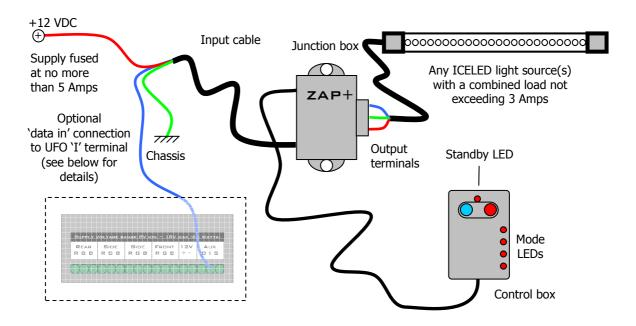
Note that other ICELED light sources e.g. TRON may also be connected in parallel with the scanner to serve as a local indication of colour and effect if the scanner is in a remote location. One scanner uses roughly half the load capacity of the ZAP+ controller so there is plenty of spare capacity for the connection of additional light sources.
