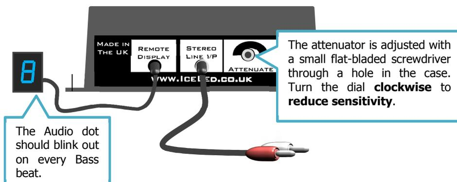
A direct line-level connection can be made to In-Car Entertainment systems using the optional link cable. This automatically disables the internal microphone so ensuring that music alone activates the light show – to the exclusion of all external sounds. The attenuator is still effective when a direct connection is used.
