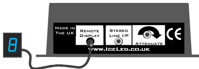
The remote-display should be positioned where the driver can see it and, as it also receives infrared commands from the remote handset, it would ideally be located at window level to allow the handset to be operated from outside the vehicle
