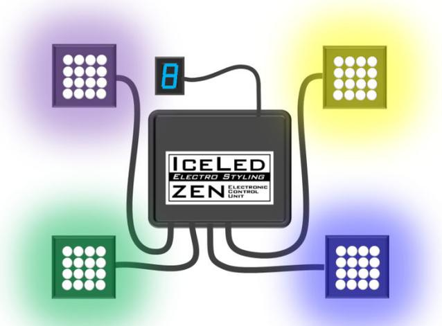
The four zones may correspond to separate areas - inside a car for example: floor; console; under-dash and roof lights.
